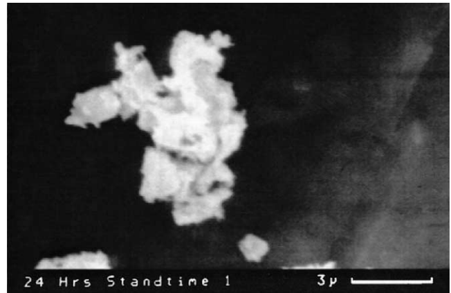
Fig. 12. High magnification image of dispersed particles as observed in the unformed positive paste after a soaking time of 24 h (magnification: 5650×).
